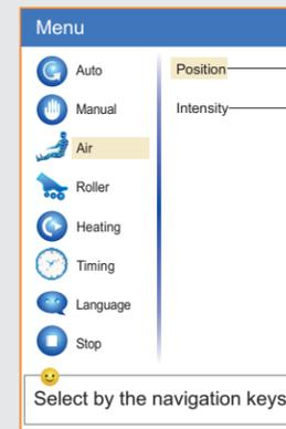
**Air** : After press MENU button, choose "air pressure" through navigation key, Press "OK" button , there are two kinds of air pressure related function: Position and Intensity; Choose the corresponding function, then press "OK" to enter next menu and choose required function.
