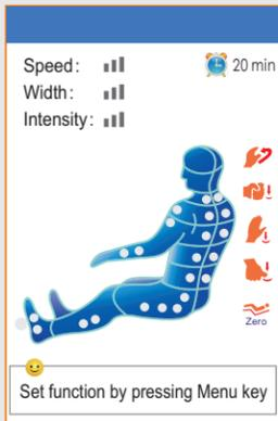
Press "on/off" button when power on, a buzzer beeps once short and brittle. LCD screen display boot screen, after 2-3 second it display the main interface and enter standby mode. Main interface show massage position, methods, time, current massage status and so on, all information will be updated timely when the chair start working.
