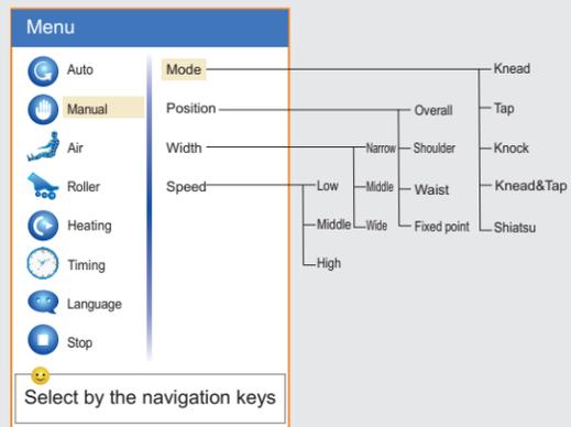
**Manual** : press "menu" key, select manual massage by the navigation key, press the "OK" button, there are four options: mode, position, width adjustment, speed adjustment : select the corresponding function, then press the "OK" button to enter the next menu, select the desired massage method, position, width and speed regulating function.
